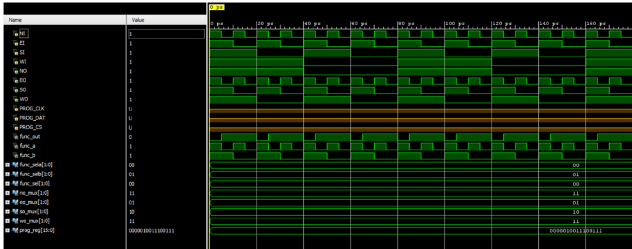
Figure 3 - EHW Cell Logic Simulation
